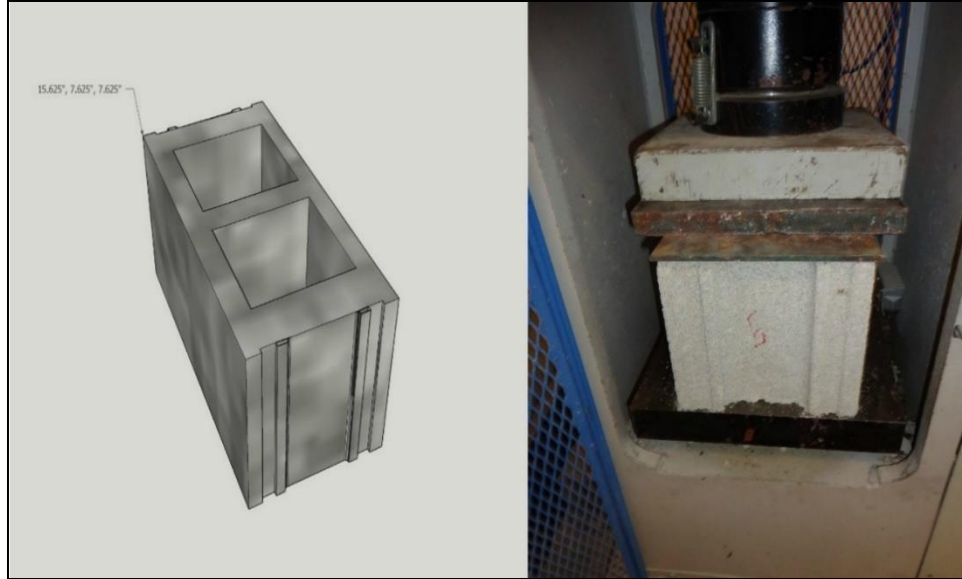
Figure 3.6 Concrete block (left) and block during compression test (right).
