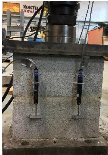
Figure 3.7 CM prism compression test setup per ASTM C1314 (ASTM 2003a).
