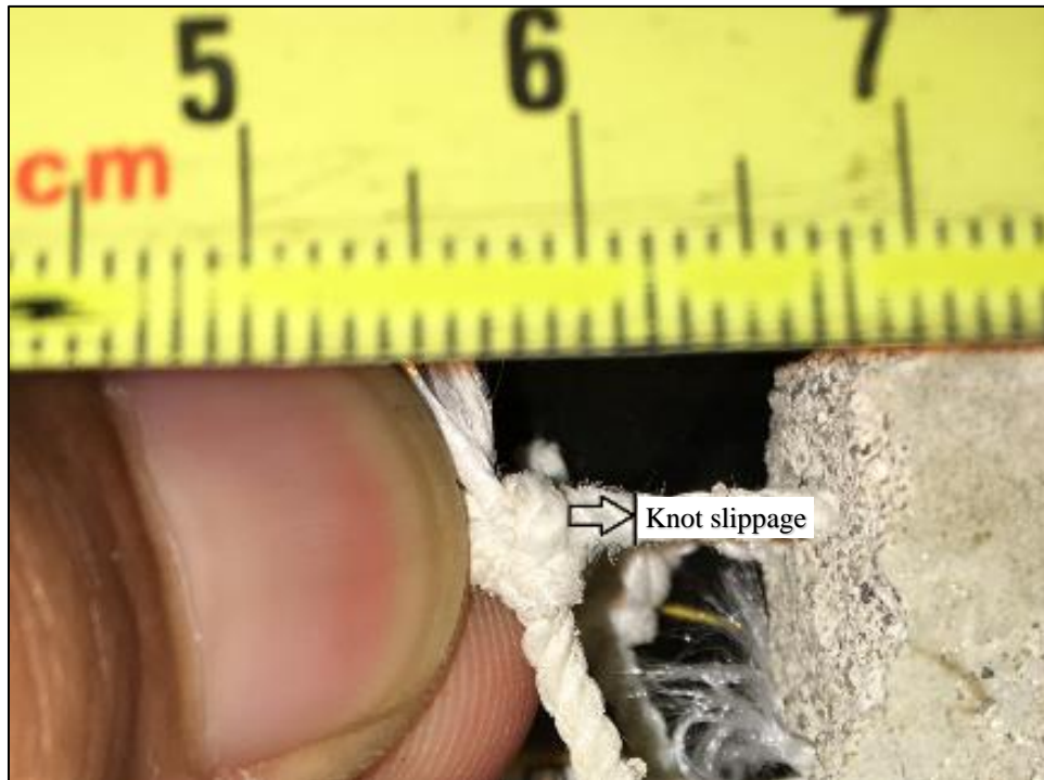
Figure 4.21 FN thread slippage from knot at cracked section.
